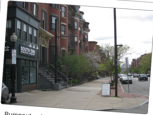
Bumpouts shorten crossing distances and provide drivers with visual clues to slow down
