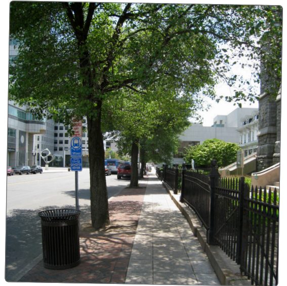
Minimum standard streetscape must include sidewalks of ample width, street trees that can mature to have a canopy, and amenities such as trash cans and benches
